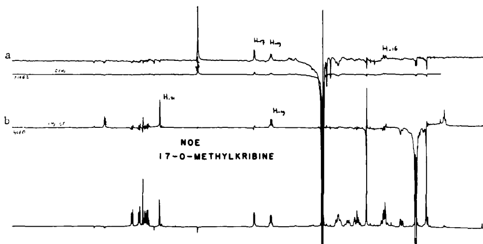
FIGURE 11. NOE-difference spectra of O -methylkribine (300 MHz, \text{CDCl}_3 ), a irradiated at OMe-signal, b irradiated at H-18
